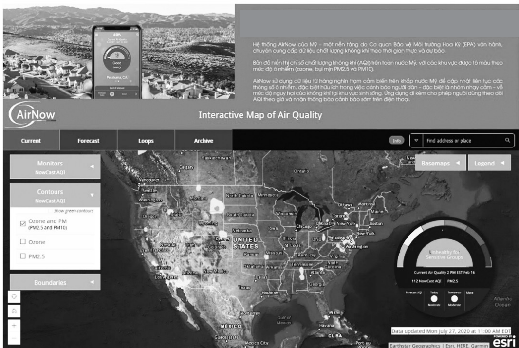
The American AirNow system collects data from more than 4.000 monitoring stations nationwide, combining AI algorithms to analyze and provide real-time AQ information
