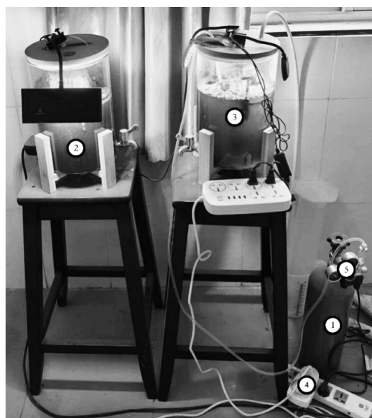
Figure 1. PhBR-B system with CO 2 source: 1- CO 2 tank, 2- The hermetic photobioreactor-biofilter (PhBR-B), 3- PhBR-B with CO 2 supply, 4-electrical systems, 5-one-way valve
